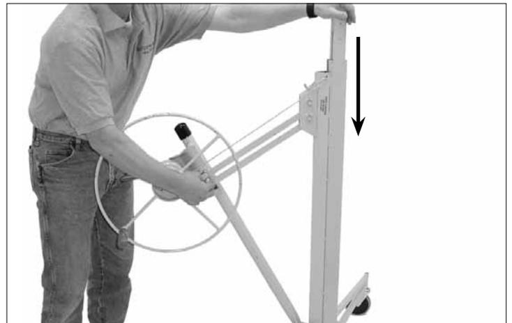
6. While holding the slide bar lock in this disengaged position with your right hand, push down on top of the telescoping section with your left hand. This action will cause the winch assembly to move toward the frame.
